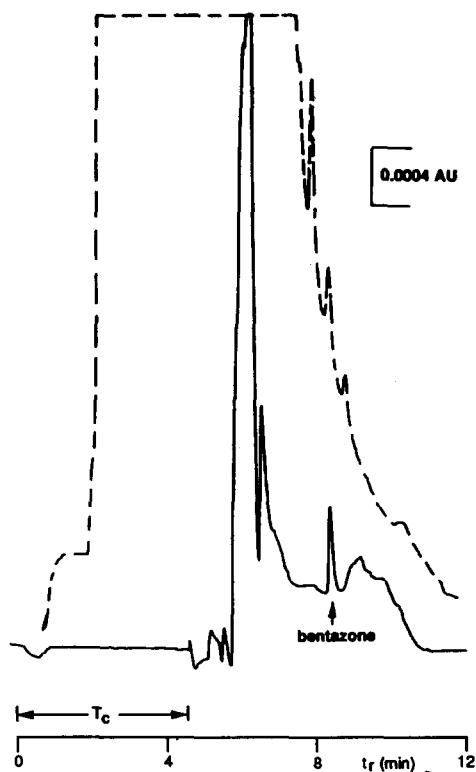
Fig. 5. RPLC-UV (220 nm) of a surface water sample containing 0.40 \mu\text{g/l} bentazone; injection volume, 2.00 ml. Solid line, chromatogram obtained with the coupled-column procedure (see Experimental section); dashed line, chromatogram obtained with the same two columns coupled on-line without column switching using a mobile phase of methanol–0.02 M phosphate buffer, pH 2.7 (50:50, v/v) at 1 ml/min; t_c , clean-up time on C-1 with coupled-column procedure.
